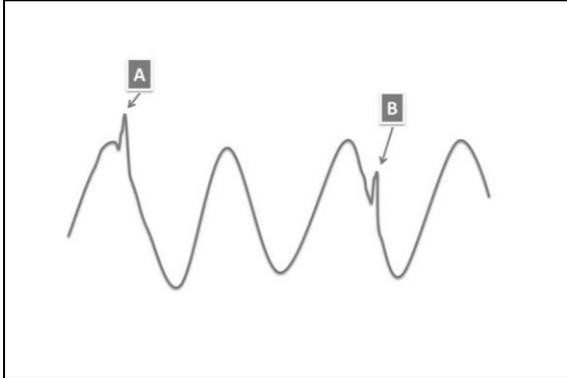
Figure 1: Hypothetical single-band signal showing 2 different types of anomalies – a spectral anomaly (A), and point anomaly (B).
