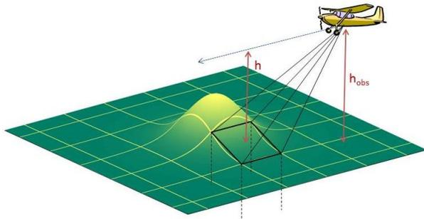
Figure 3: Schematic showing the parameterization of the topography using prism sources with slanted top surfaces relative to the detector.
