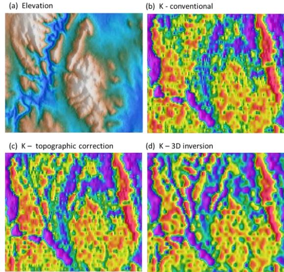
Figure 5: Pseudo-colour images from the SE Lachlan survey area: (a) digital elevation model, (b) K concentration (%) gridded using minimum curvature (c) K concentration (%) after topographic correction - gridded using minimum curvature, and (d) K concentration gridded using 3D inversion. The images are centred on (149:04:39.99 E, 35:40:25.74 S) and are about 15 km wide. Data courtesy of the Geological Survey of NSW.
