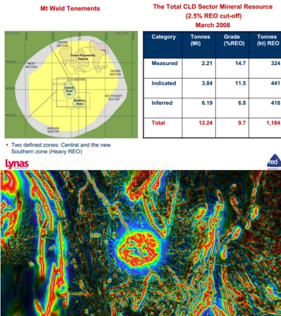
Figure 7: Mt Weld rare earth oxide deposit. (a) schematic plan, (b) mineral resources, (c) magnetic response, with rtp, drape tilt angle. Data courtesy of the Geological Survey of WA.
