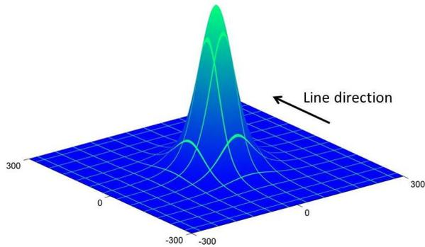
Figure 4: Source-detector response for a slab detector at 60 m height above a vertical rectangular prism source centred at (0,0) with dimensions 50x50 m. The figure is 600 m wide in the x and y dimensions.
