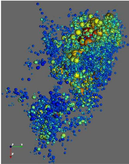
Localisation of micro-seismic events : **3200m x 1800m** horizontally (long-axis oriented NNE) and within **600 m** vertically.
