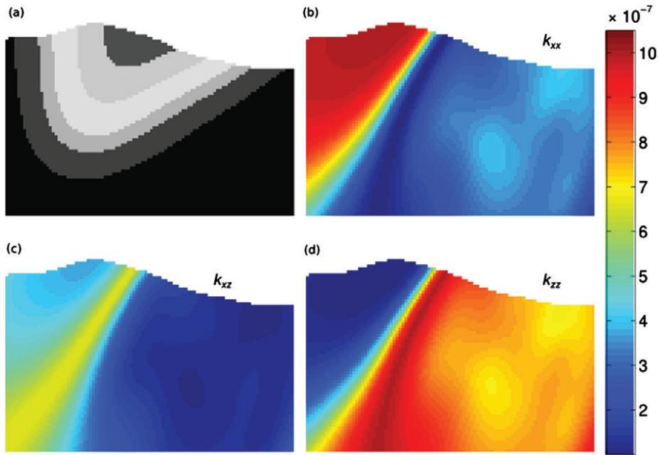
Figure 1. (a) Geological model: a perched syncline. The lithology is assumed to be uniform but folded, the colors represent only the age of the formation; (b)  $k_{xx}$  component of the hydraulic conductivity tensor; (c)  $k_{xz}$  component, (d)  $k_{zz}$  component. The color scale is given in [m/s] and is relative to b, c, and d subfigures.
