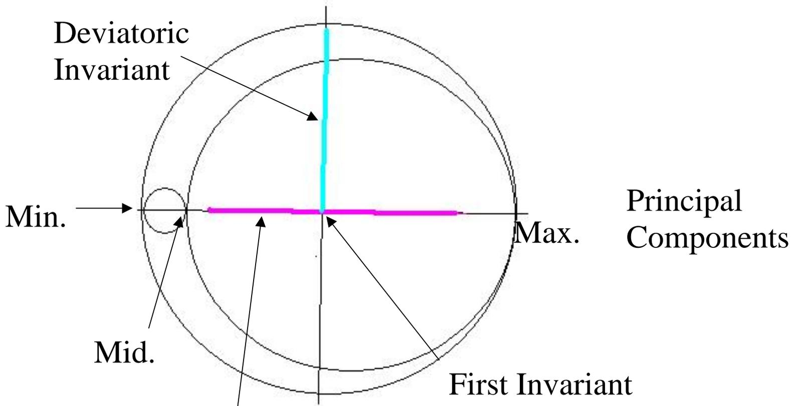
In the case of gravity gradiometry, the First Invariant of the tensor is supposed to be zero, and so a vertical axis is shown at this point. The tensors are symmetric, so only the top half need be shown. The horizontal axis represents the normal or principal components and the vertical axis represents the rotational gradients.
