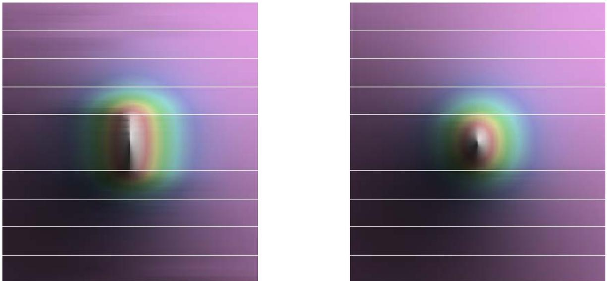
The left image is standard gridding and the right image shows gradient enhanced gridding. The missing observation line is used to stress test the algorithm.
