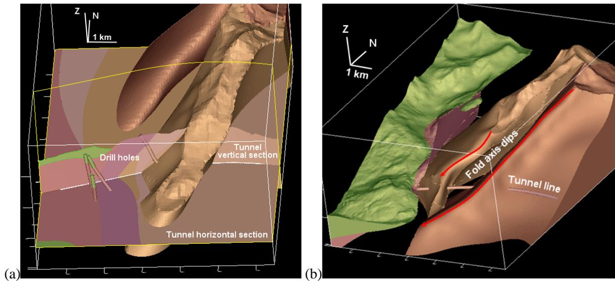
Fig. 3. 3D Model of the Sapey-Orgère zone (Alps). (a) View from South. Plane and curved sections along the tunnel are derived from the model. (b) View from S-E. Uncertainties along the tunnel are inferred by changing the interpretation of fold axis dips.
