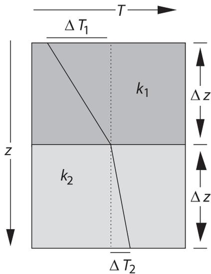
Figure 5. Cartoon illustrating how the geothermal gradient changes with depth if a low conductivity layer ( $k_1$ ) overlies a high thermal conductivity layer ( $k_2$ ). This is a special case of what is more generally known as heat refraction. Source: Stüwe 2007
