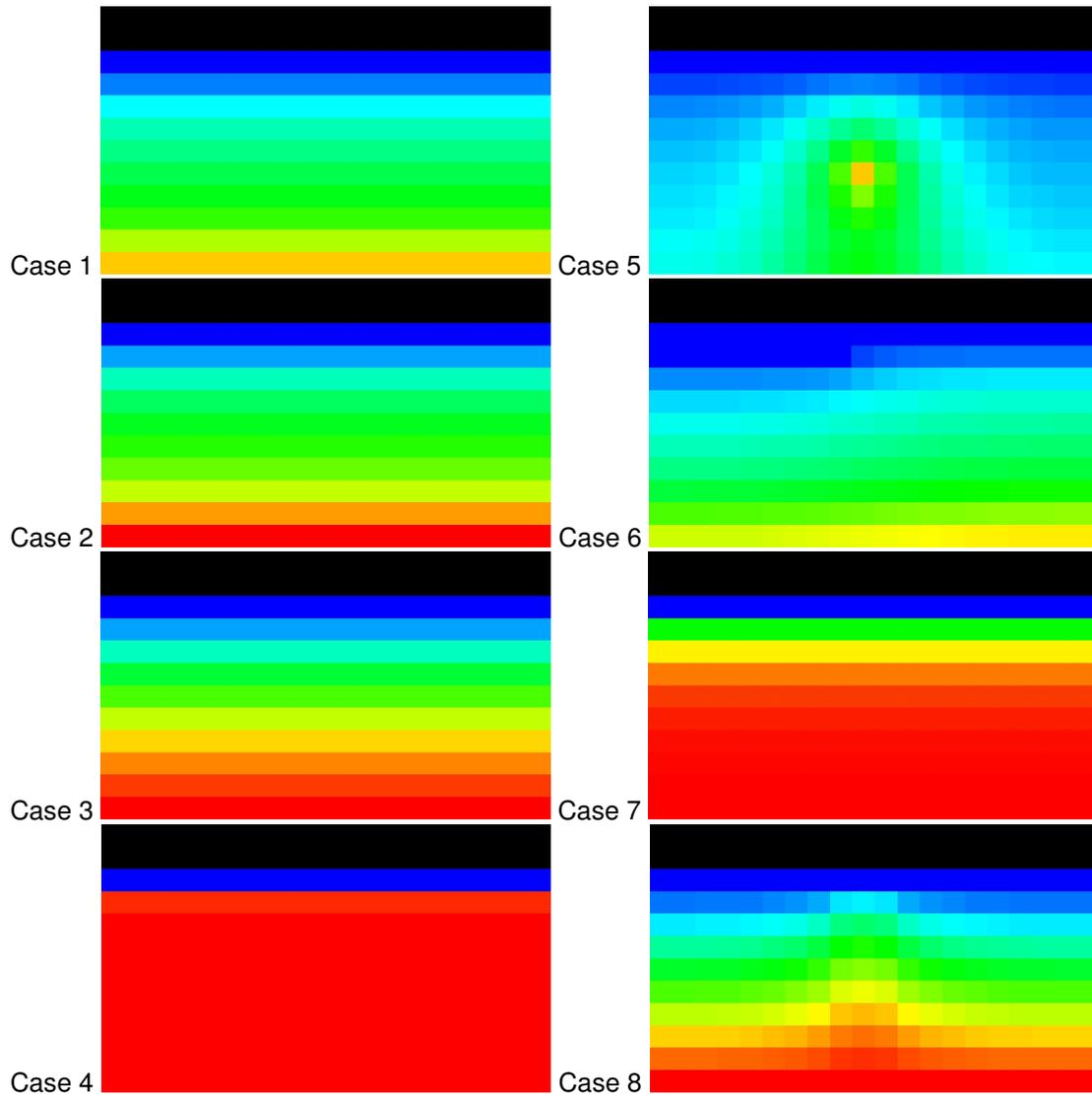
Figure 3. Unit test results for Cases 1 to 8: 2D sections rendered from 3D solutions predicting temperature variation for each case. See Table 2 and Fig. 2 for case details. Legend details: Red is maximum and blue is minimum, colours between are at linear intervals. For Cases 1, 4 and 6 the temperature range is 0 to 6 °C; for Cases 2, 3, 7 and 8 the temperature range is 0 to 100 °C; and for Case 5 the temperature range is 0 to 50 °C.
