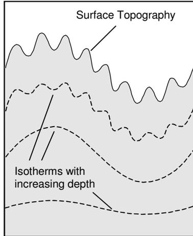
Figure 1. The influence of surface topography on isotherms at depth (after Stüwe K. and Hintermüller M., 2000)
