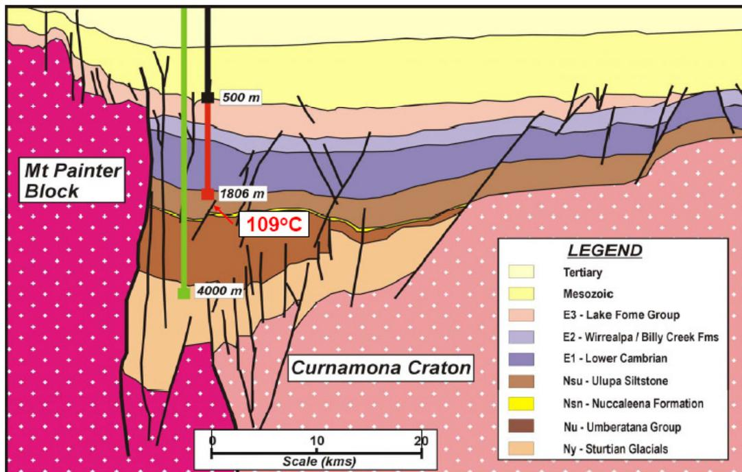
Figure 4. Generalised west-east cross-section through the Poontana Graben, northern Flinders Ranges, South Australia. E1 - E3 are sedimentary rocks of the Cambrian Arrowie Basin; Nsu, Nsn, Nu, Ny are sedimentary rocks of the Pre-Cambrian Adelaidean sequence (source: Petratherm Ltd.)
