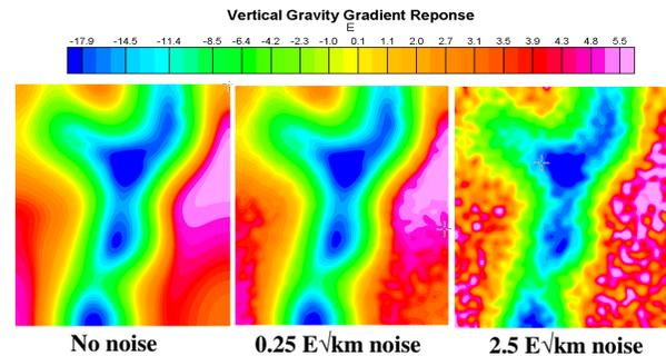
Figure 3. Vertical gravity gradient ( $G_{zz}$ ) response simulated for an airborne survey flown at 150m ASL. The no-noise, 0.25  $E\sqrt{km}$  noise and 2.5  $E\sqrt{km}$  noise are shown. The noise added  $G_{zz}$  responses have been filtered with a 2000m low-pass filter.
