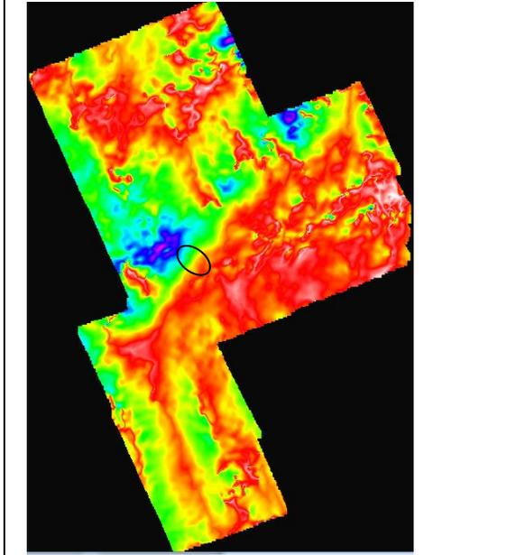
Figure 6 Montezuma gridded tensor data with a phase enhancement derived from rotating each tensor to solve the Eigen system (hence like an AGC filter). The NE cross-cutting fault and the N20W rift bounding faults are clear. Ellipse shows approximate working point for most of this study.
