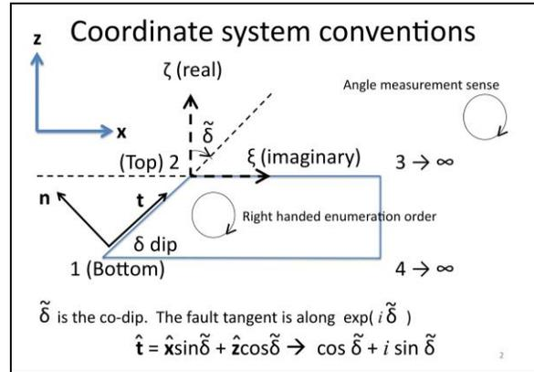
Figure 1. Fault geometry and reference systems.
