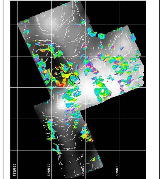
Figure 7 Montezuma vertical gravity greyscale, 3 levels of upward continued multiscale edge picks or worms, and the full tensor eigensystem derived strike vectors, showing the zones where a 2D signal character dominates the observed signal.
