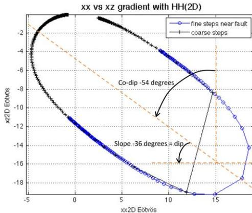
Figure 4 Components  $xx$  and  $xz$ , plotted against each other, form a segment of a closed oval curve, rotated by the co-dip angle.
