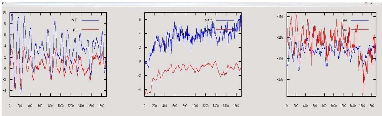
**Figure 4. The two measures of the Euler angles from the system. The Blue is from the INS before Kalman filtering and the Red is estimated from the B field and acceleration vector. Note the separation in the estimates as well as the amplitude differences.**
