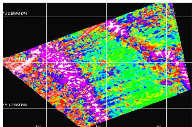
**Figure 3. Part of a magnetic tensor survey, partially processed, assuming the attitude is correctly estimated by the INS. The signal is the cube root of the second invariant of the tensor with units in nT/m. The clearly visible striping is reminiscent of traditional heading errors**
