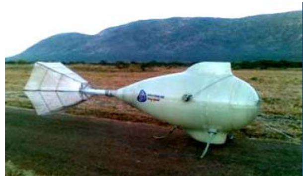
**Figure 2. Current generation towed bird for the magnetic tensor system developed jointly by Spectrem and IPHT**
