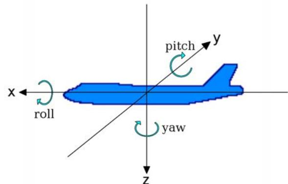
**Figure 1. Schematic showing Euler Angles, Roll, Pitch and Yaw**
